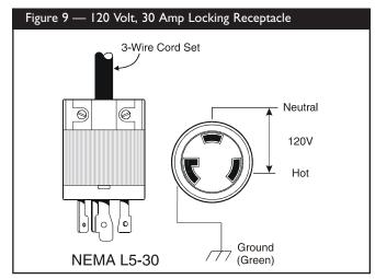
Use this receptacle to operate 120 Volt AC, 60 Hz, single phase loads requiring up to 3,600 watts (3.6 kW) of power at 30 Amps. The outlet is protected by a 30 Amp push-to-reset circuit breaker.
